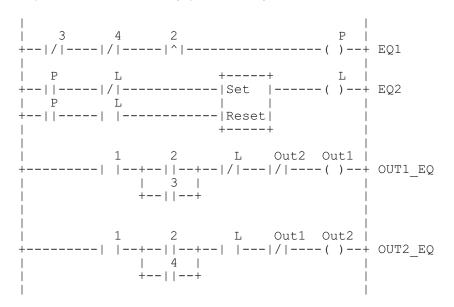
Rung P is equation 1. It generates the pulse that will toggle the latch. The pulse comes from the RISE function.
